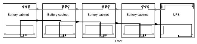
1. Route the battery breaker trip cable from J1 in the first modular battery cabinet to J3 in the next modular battery cabinet. Repeat the procedure for all modular battery cabinets.
