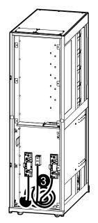
4. Connect the ground cable first, and then connect BAT+, BAT-, and CT (midpoint) cables between the modular battery cabinets in a daisy chain.
