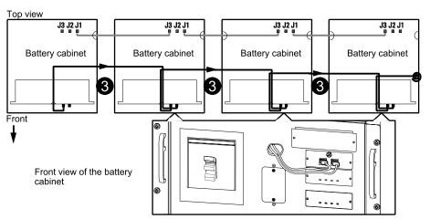
4. Route the communication cable from XR Communications port 1 in the last modular battery cabinet to the UPS XR Communications port 2.
