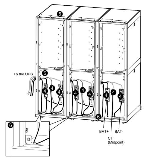
5. Route the ground cable and the BAT+, BAT-, and CT (midpoint) cables from the first modular battery cabinet to the UPS through the side, top, or bottom of the modular battery cabinet.
