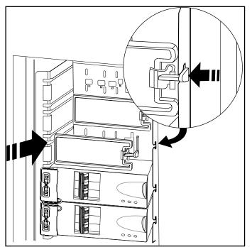
11. Install the slot lock by pressing it into the slots.
