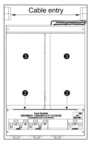
3. Remove the two cover plates by sliding them towards the middle of the cabinet and lifting.
