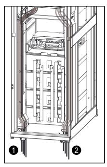
2. Route the input and bypass cables (if applicable) from the bottom through the cable conduit in the right side (seen from the rear) to the cable landing area.
