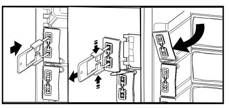
4. To remove a filler plate: Press down on the filler plate clip to release the locking mechanism and pull the filler plate directly towards you.
