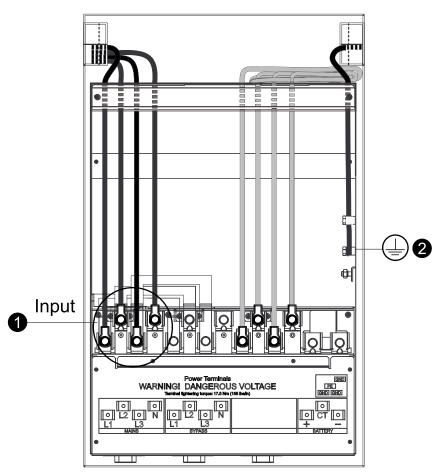
2. Connect the Protective Earth (PE) cable.
