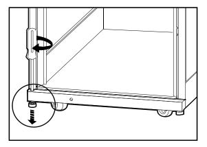
2. Use a wrench to adjust the four leveling feet and ensure that the cabinet is level.
