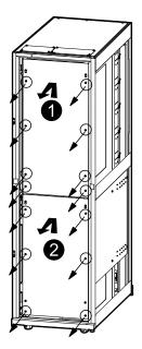
2. Loosen the two top bolts and remove the eight lower bolts from the lower cover plate. Lift the plate to remove it.
