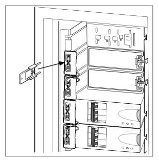
2. Squeeze the sides of the key inwards to grasp the slot lock firmly.
