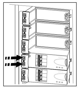
12. Connect the power distribution module cable to the appropriate equipment.
